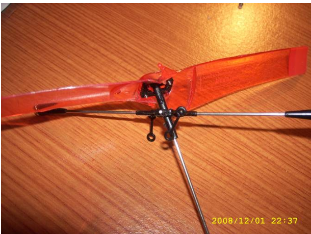
10) Unhook the I-chain that is hooking onto the top rotor.
