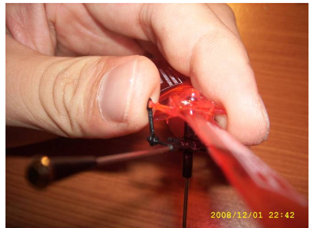
13) Secure back the I-chain and the two screws on the top rotor.
