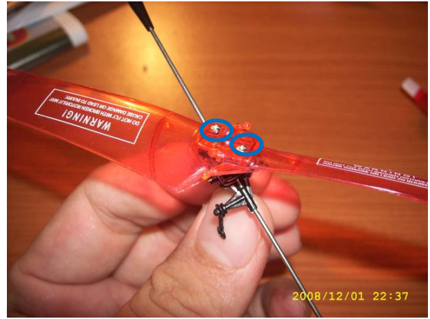
11) Remove the two screws.
