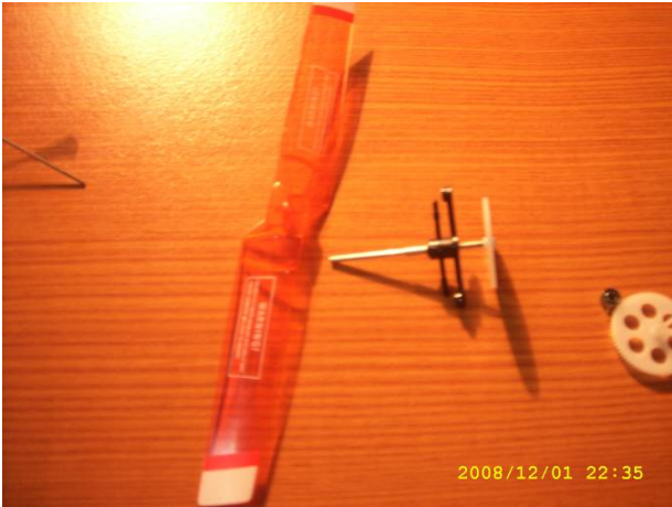
9) Remove and replaced the bottom rotor.
